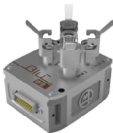
WB Node with 2 vibration sensors + 2 rpm sensors
